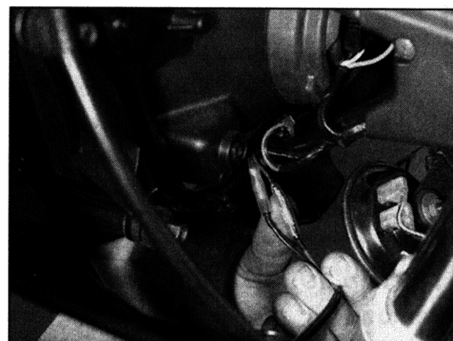
5.11c ... and the turn signal wiring connectors
