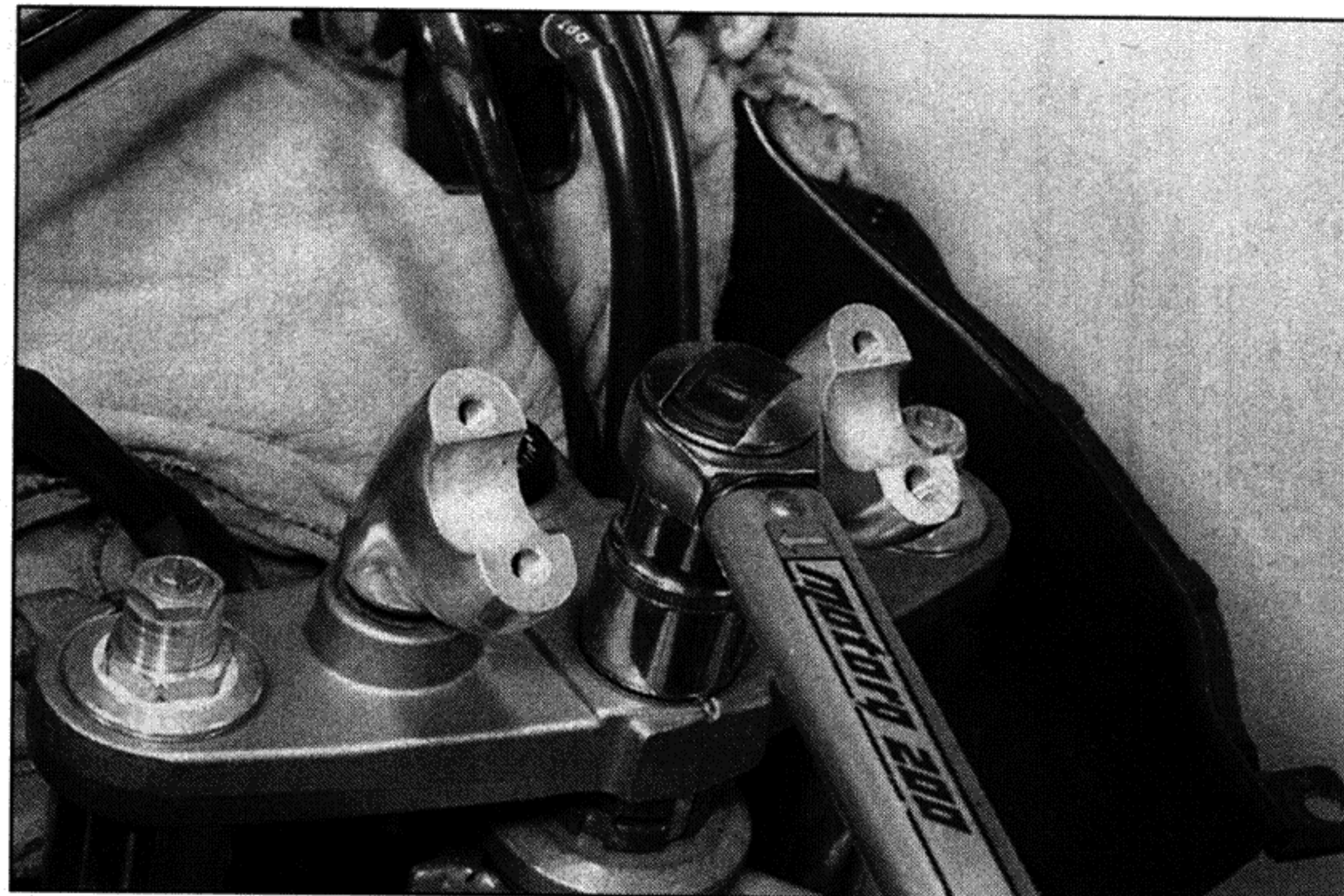
8.13 Tighten the steering stem nut or bolt to the specified torque
