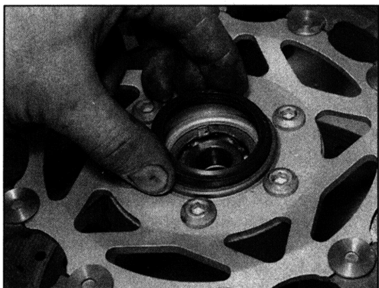
13.13 Press the grease seal into place
