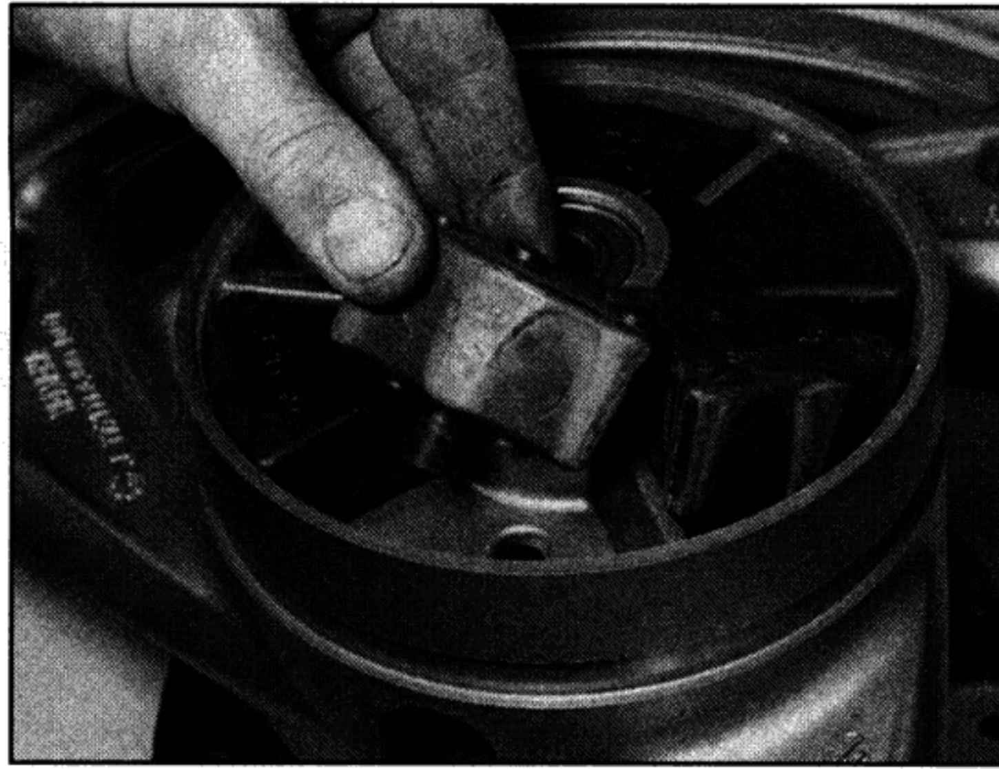
17.3 . . . and remove the rubber dampers
