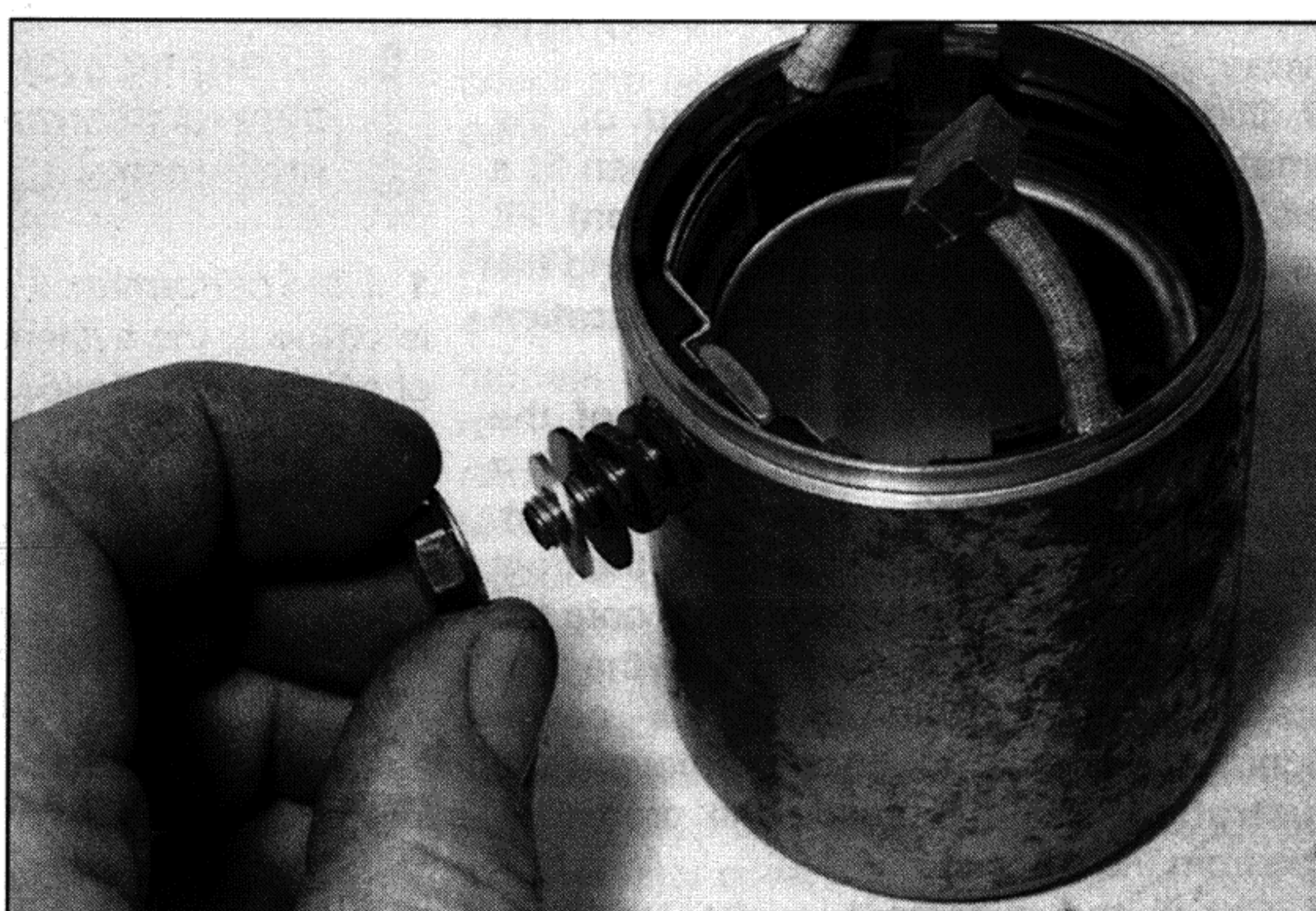
29.15d . . . and fit the washers and nut
