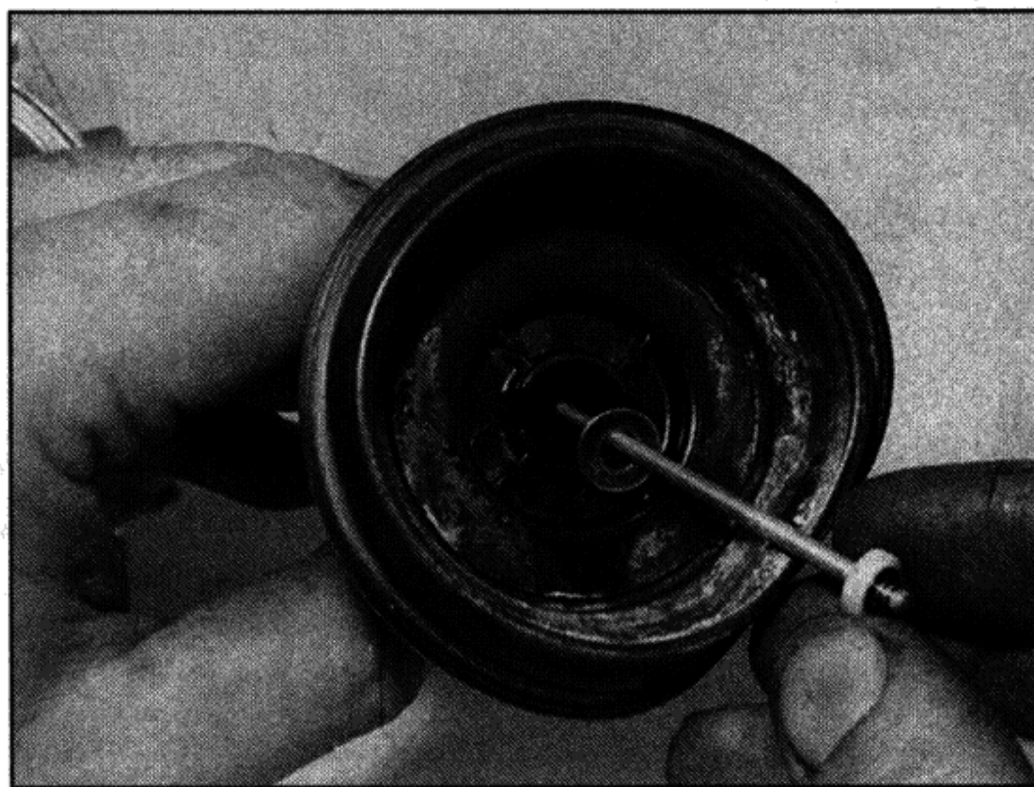
8.5 Remove the jet needle and its washer
