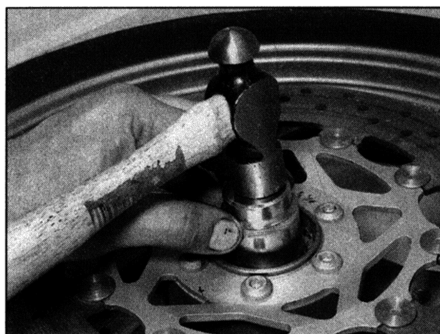
13.10 A socket can be used to drive in the bearing
