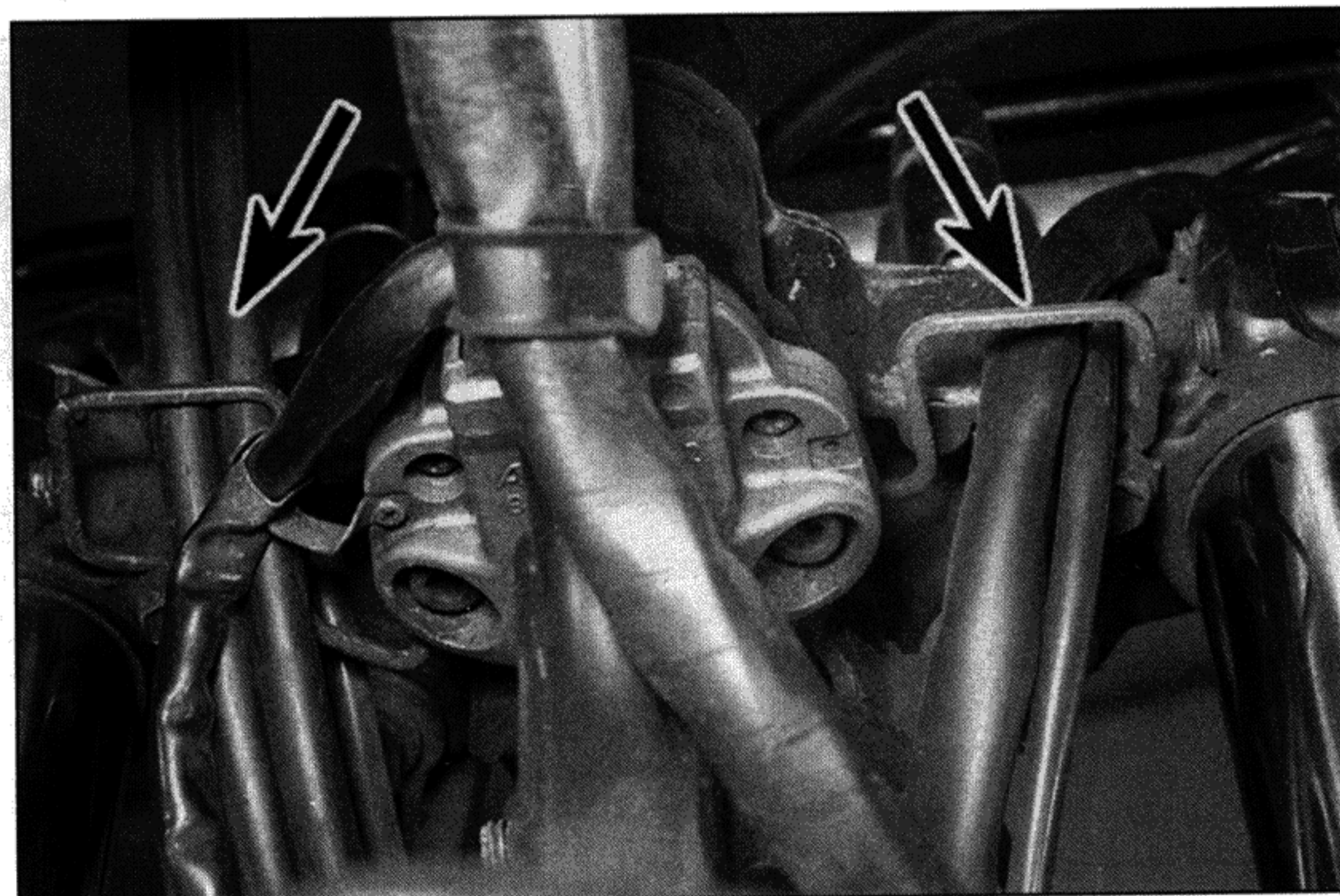
8.4a Free the cable and wiring from the guides (arrowed) on the top yoke . . .
