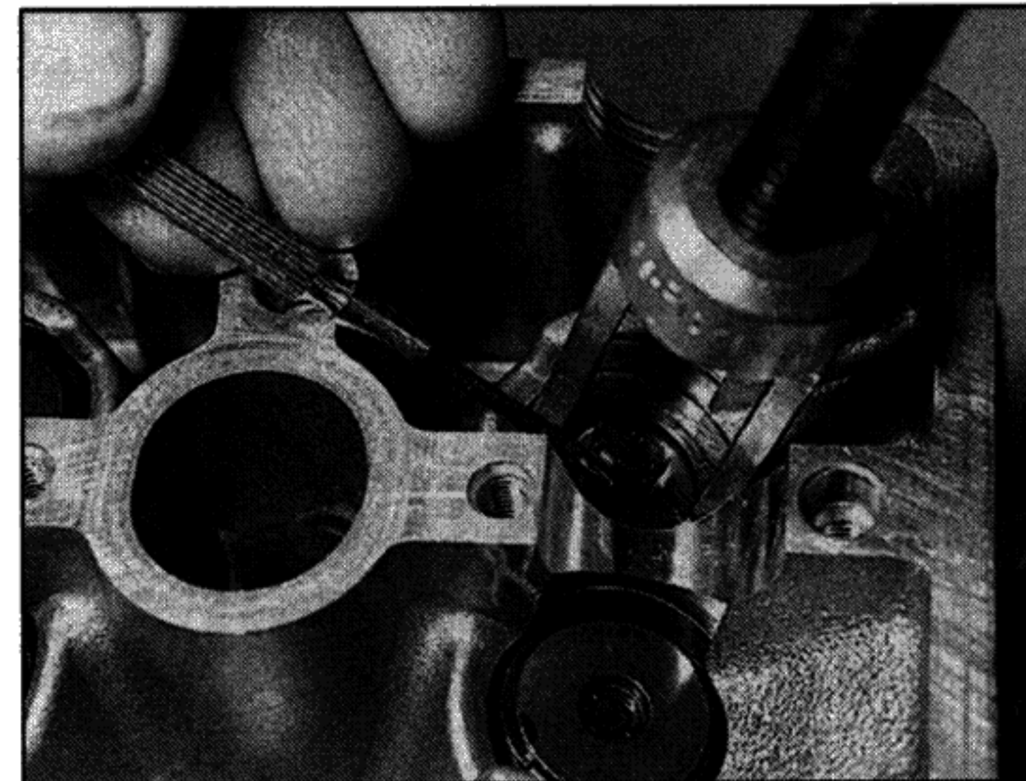
12.27b Compress the spring and install the collets, making sure they locate in the groove
