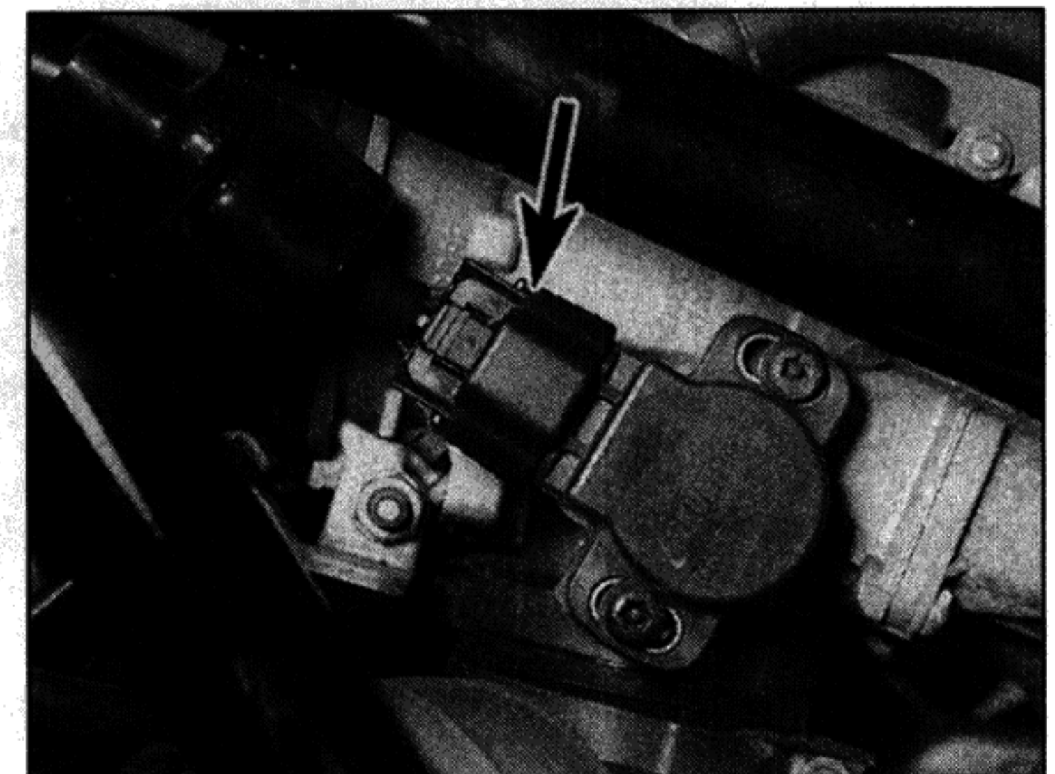
7.6 Disconnect the throttle position sensor wiring connector (arrowed)
