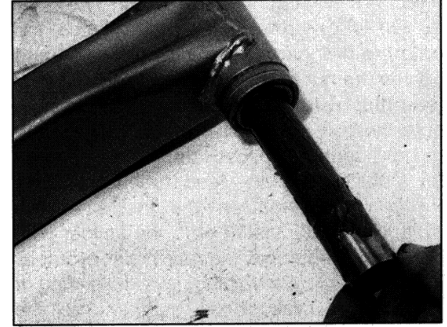
13.14b ... then withdraw the collar ...
