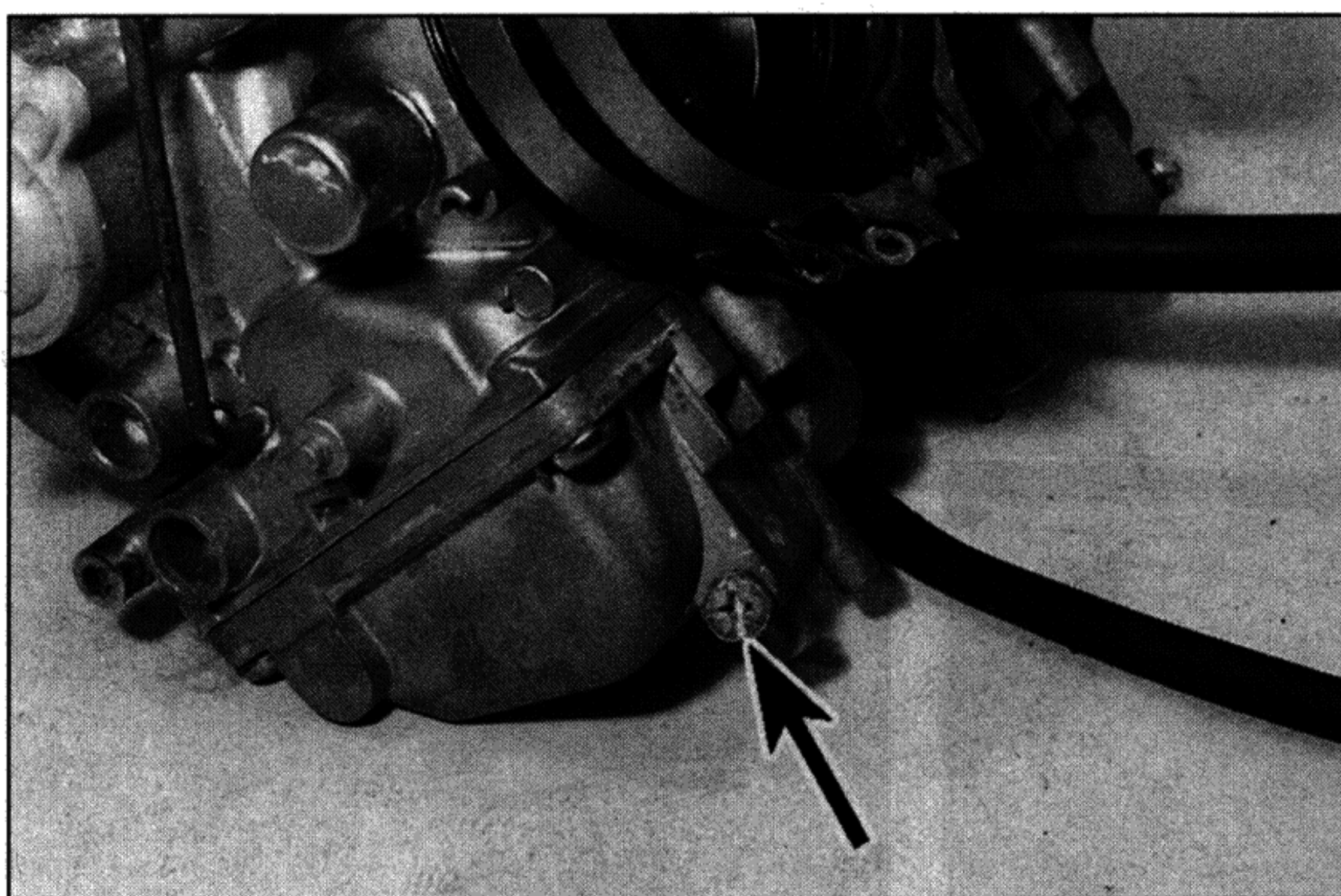
7.8 Float chamber drain screw (arrowed)
