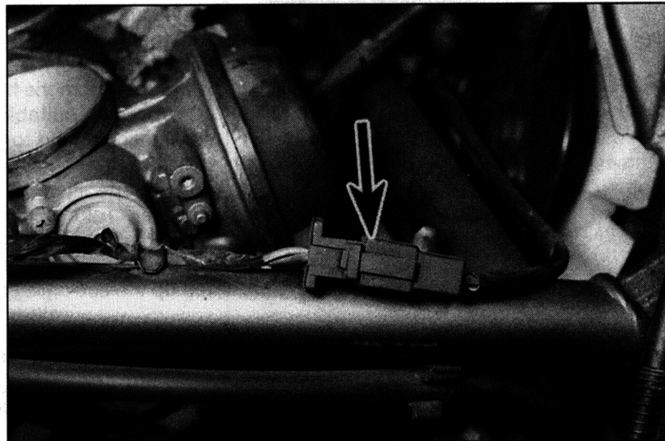
4.3b Fan motor wiring connector (arrowed) – XTZ models
