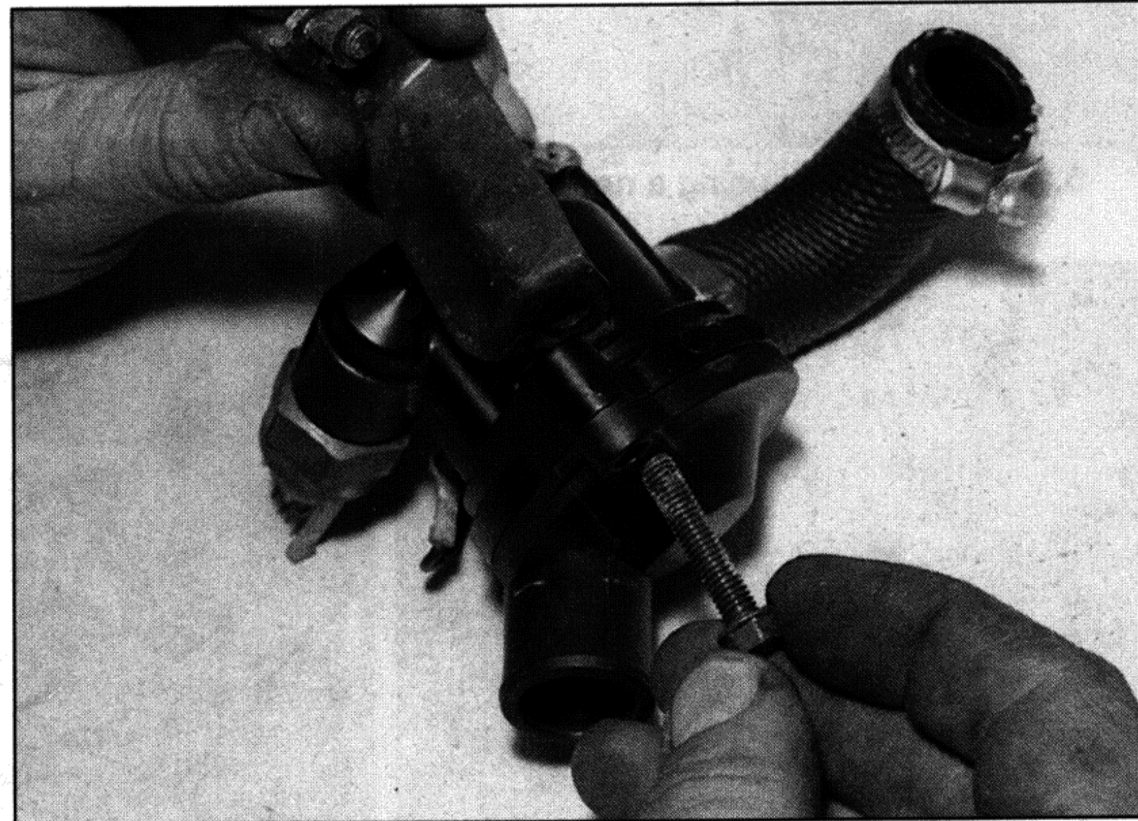
6.6a Unscrew the bolts and remove the cover . . .
