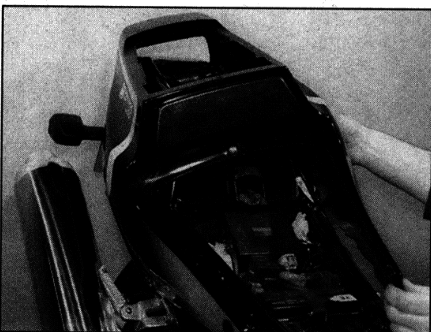
3.5b ... and remove the side cover assembly
