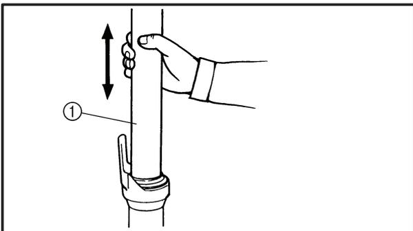
9. Slowly stroke the inner tube ① up and down.
